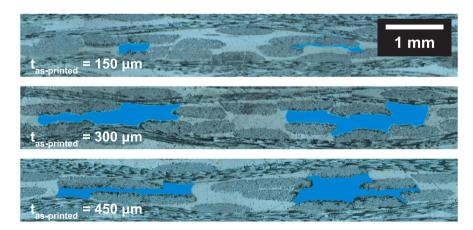
Figure. A.1. EMAA thickness variation. Tiled optical micrographs of GFRP composite cross-sections for 24% EMAA at varying as-printed thicknesses (150, 300, and 450  $\mu$ m) showing different EMAA melt-bonding morphologies (blue overlay) resulting from respective placement between fiber-tows.
